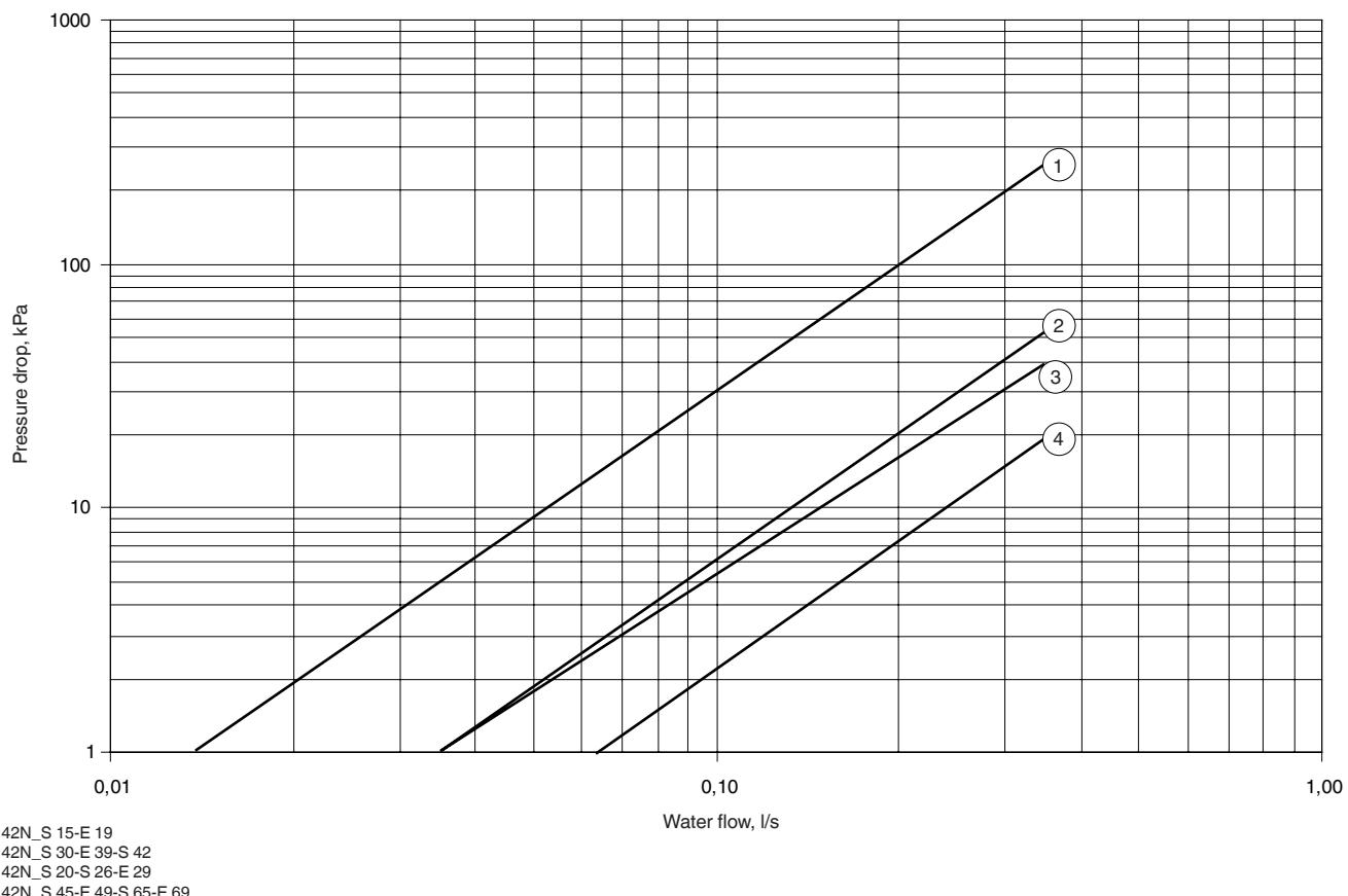
Heating conditions (entering water temperature = 50°C)
