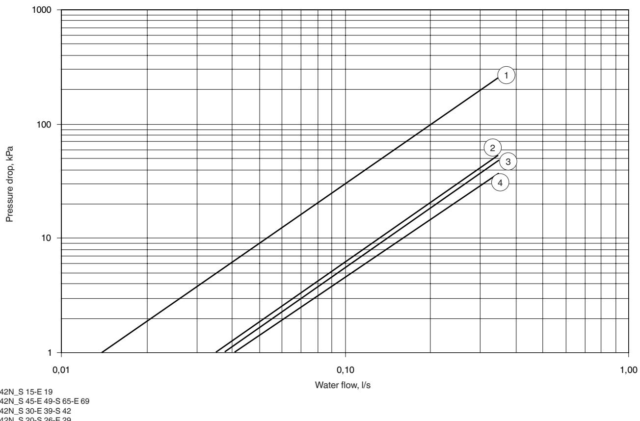
Heating conditions (entering water temperature = 70°C)
